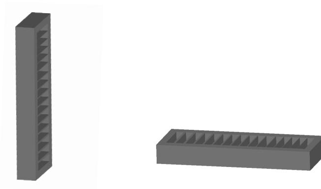
**Figure 1:** Via the left side orientation, the walls are horizontal with relation to the surface of the build where the build top is located at the uppermost surface; therefore this orientation will be referred to as the horizontal orientation. Via the orientation shown on the right, the internal walls are vertical in relation to the surface of the build therefore this orientation will be referred to as the vertical orientation.
