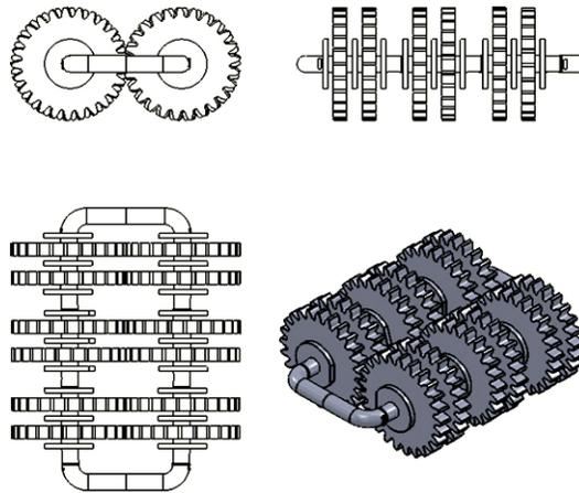
**Figure 6:** This gear was designed to test how much the center distance can be varied before fusing occurs and or before the gears fail to mesh during rotations. The three gear pieces test separate sizes with 15-20 teeth. Gear pairs run the length of the design. The center distance is gradually increased by 0.5 mm.
